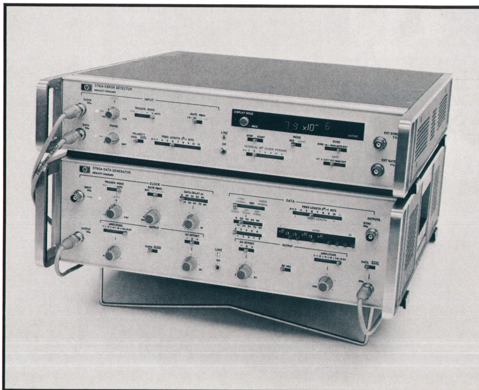
Fig. 1. Model 3760A Data Generator (lower unit) supplies a variety of bit patterns that are useful for testing digital systems and logic operations. Model 3761A Error Detector detects errors introduced into the data generator's pseudorandom sequences by equipment under test, and measures the rate at which errors occur.
